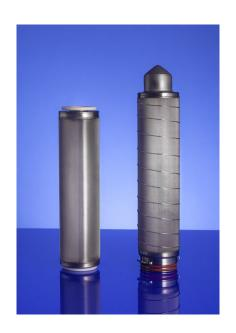
Filter elements are made with wire meshes and cloths supported by a high-strength stainless steel core (slotted screen); the ends available in SOE and DOE configurations are welded to the core. The "SOLINOX" filter elements can be regenerated by mechanical action, backwashing, chemical or ultrasonic cleaning.
